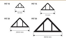
**LAYING INSTRUCTIONS**Put the nails into the central part along the profile before pouring the concrete.
