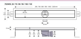
DUCT BODY MADE OF AISI 304 STAINLESS STEEL
